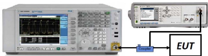
Figure 7-7. Test Instrument & Measurement Setup
