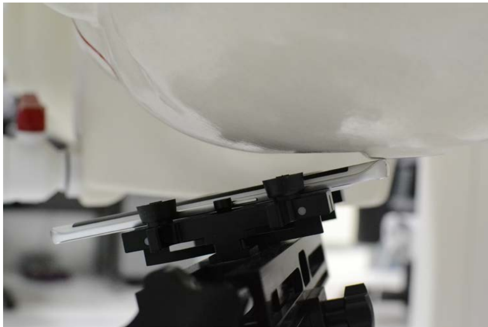
SAR Test Setup Photo 4 – Left Tilt
