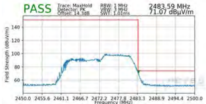
Plot 7-168. Radiated Restricted Upper Band Edge Measurement SISO ANT1 (Peak - 106 Tones)
