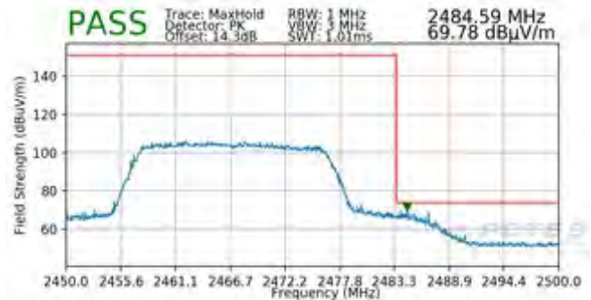
Plot 7-178. Radiated Restricted Upper Band Edge Measurement SISO ANT1 (Peak - 242 Tones)
