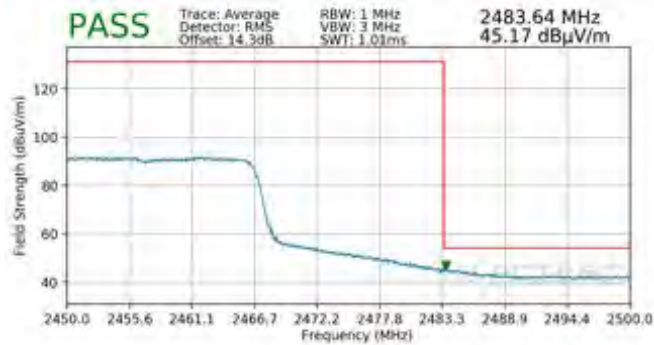
Plot 7-217. Radiated Restricted Upper Band Edge Measurement MIMO (Average – 242 Tones)
