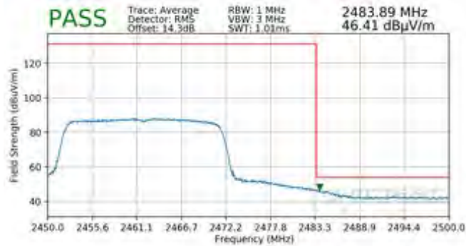
Plot 7-181. Radiated Restricted Band Edge Measurement SISO ANT1 with WCP (Average – 242 Tones)
