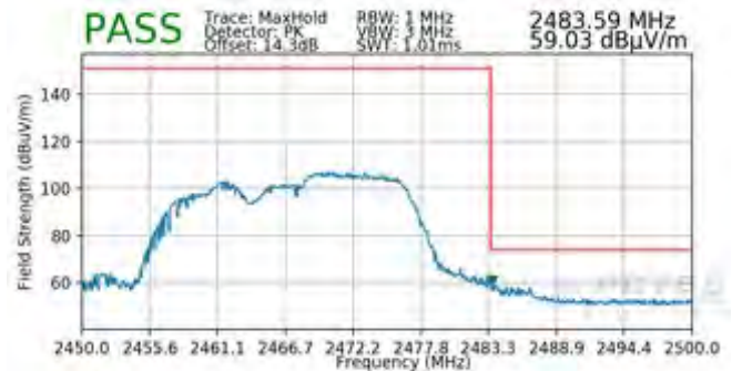
Plot 7-210. Radiated Restricted Upper Band Edge Measurement MIMO (Peak - 106 Tones)
