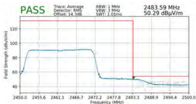
Plot 7-197. Radiated Restricted Upper Band Edge Measurement SISO ANT2 (Average – 242 Tones)
