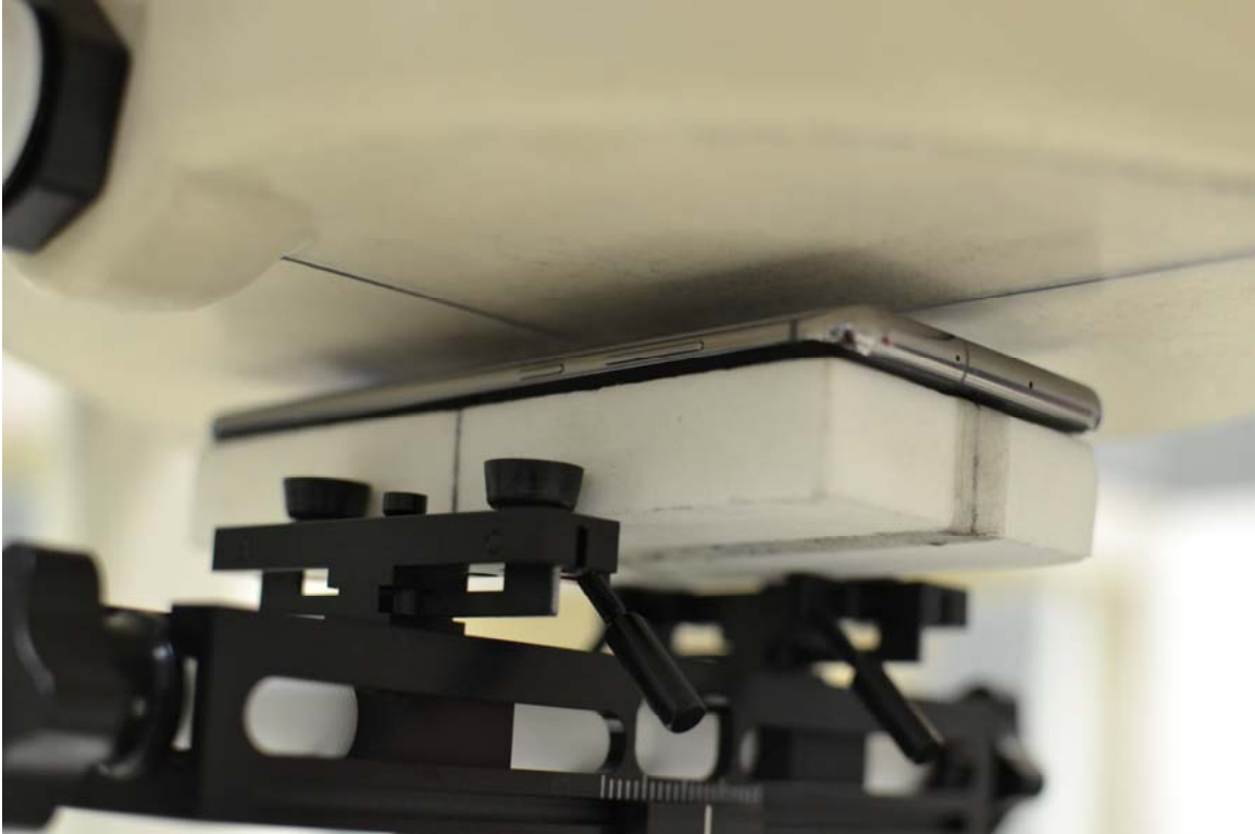
SAR Test Setup Photo 8 – Back Side at 7 mm
