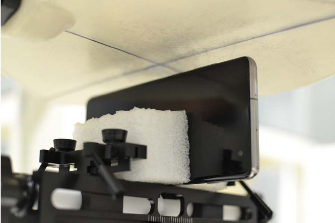
SAR Test Setup Photo 20 – Left Side at 10 mm
