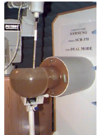
Figure 1. SAR Test Set-up
