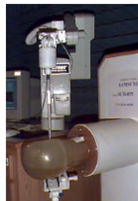
Fig. 1 SAR Test Setup
