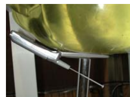
Figure 14.9 Left Head SAR Test Setup -- Cheek / Touch Position --
