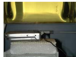
Figure 14.13 Body SAR Test Setup -- w/o Holster --
