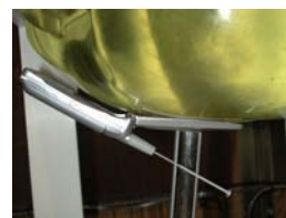
Figure 14.5 Left Head SAR Test Setup -- Cheek / Touch Position --
