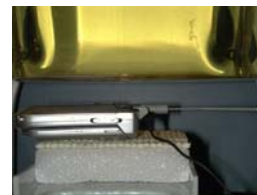
Figure 14.13 Body SAR Test Setup -- w/o Holster --
