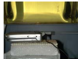
Figure 14.11 Body SAR Test Setup -- w/o Holster --
