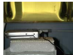
Figure 14.12 Body SAR Test Setup -- w/o Holster --
