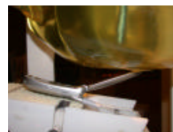
Figure A.12 Left Head SAR Test Setup -- Ear / 15° Tilt Position --
