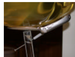
Figure A.9 Right Head SAR Test Setup -- Cheek / Touch Position --
