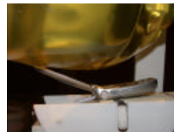
Figure A.10 Right Head SAR Test Setup -- Ear / 15° Tilt Position --
