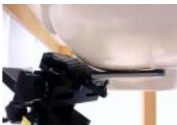
Figure 8.8 Left Head SAR Test Setup -- Cheek / Touch Position--
