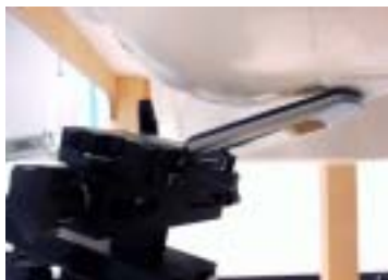
Figure 8.5 Left Head SAR Test Setup -- Ear / Tilt 15° Position --
