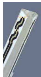
Figure 4-2 Probe Thick Film Technique
