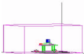
Figure 3-1. Shielded Enclosure Line-Conducted Test Facility
