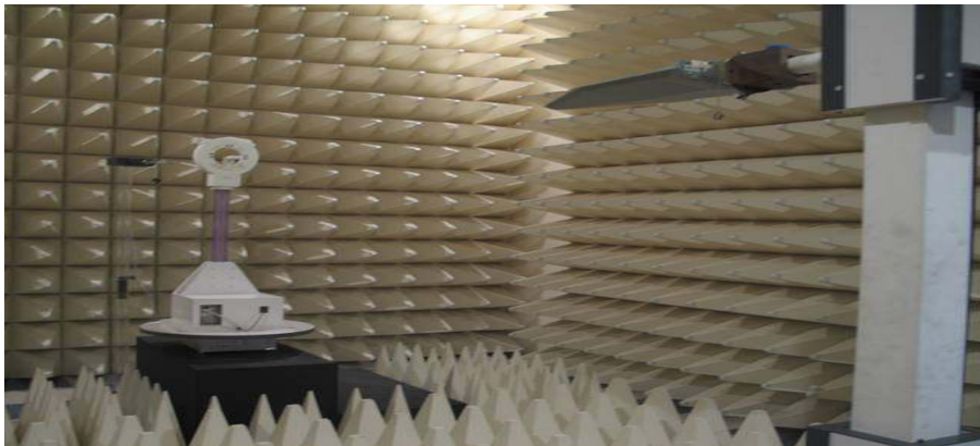
Figure2. Photograph of 3m Fully-Anechoic Chamber
