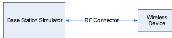
Figure 11-1 Power Measurement Setup
