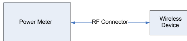
Figure 12-1 Power Measurement Setup
