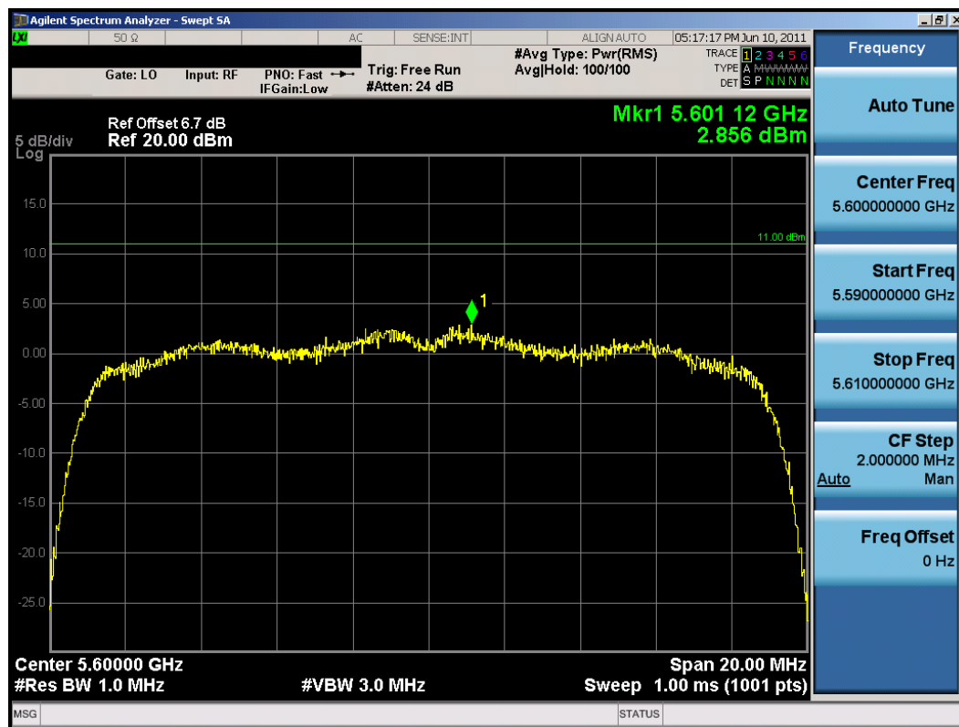
Plot 6-35. Peak Power Spectral Density Plot (802.11n (UNII Band 3) – Ch. 120)
