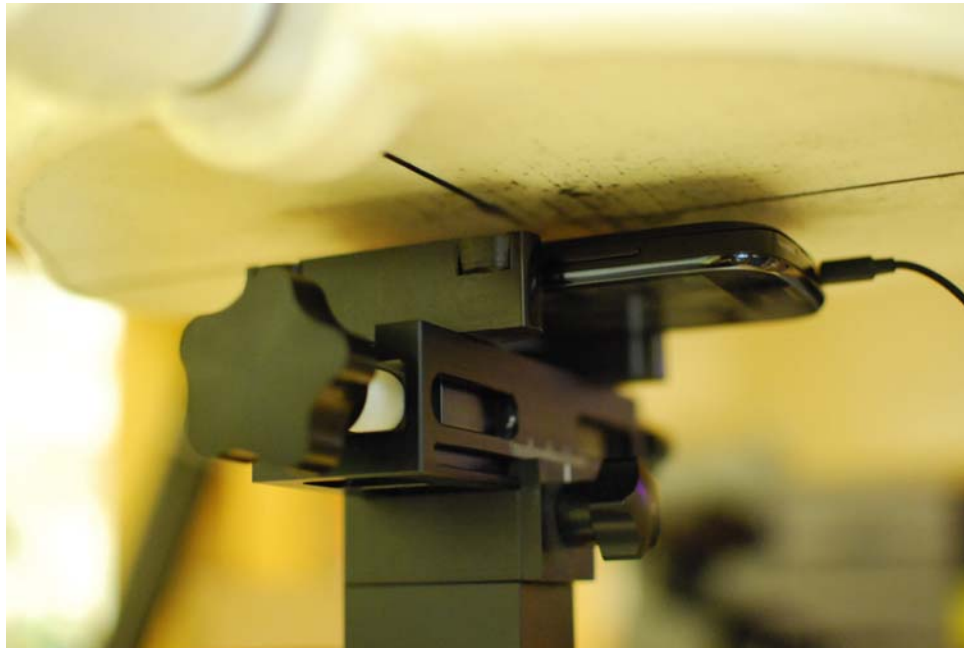
SAR Test Setup Photo 10: Body-Worn at 1.0 cm
