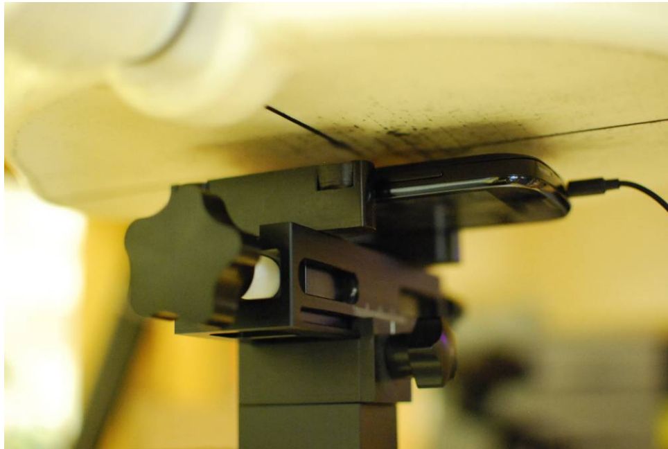
SAR Test Setup Photo 8: Body-Worn at 1.0 cm
