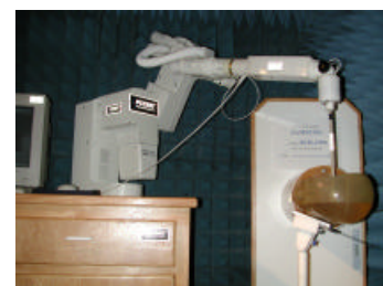
Fig. 1 SAR Test Setup
