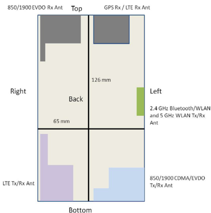
Figure 12-1 Identification of Sides/Edges for SAR Testing (Back View)
