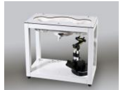
Figure 6-1 Twin SAM SAR Phantom
