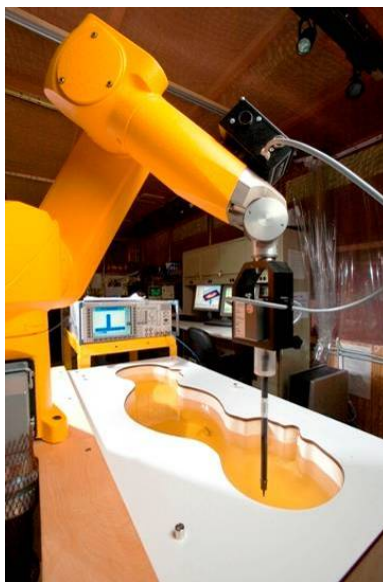
Figure 4-2 SAR Measurement System
