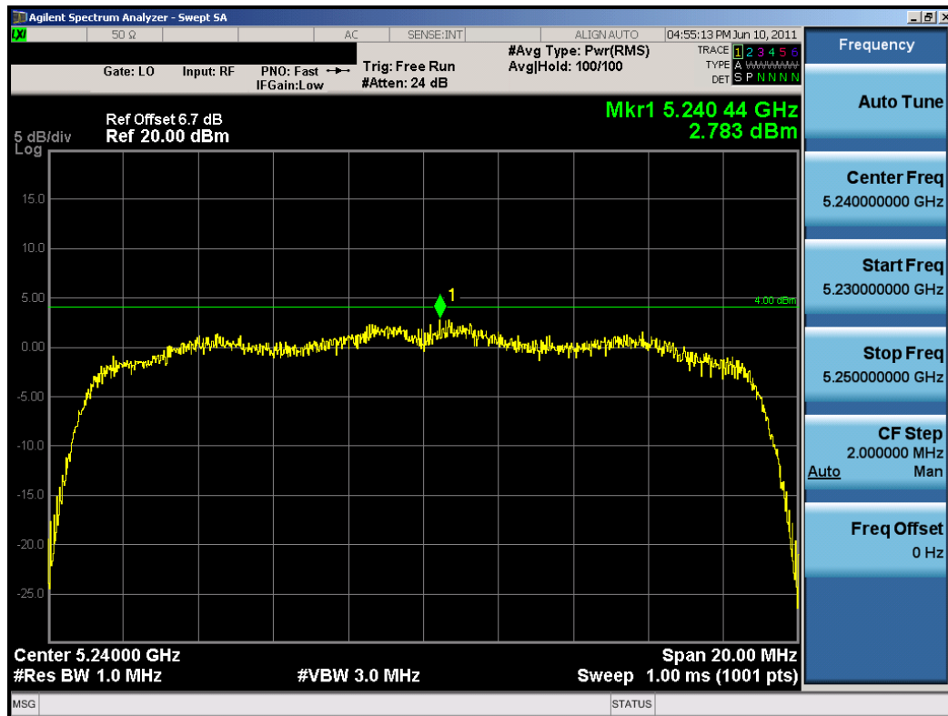
Plot 6-24. Peak Power Spectral Density Plot (802.11n (UNII Band 1) – Ch. 48)
