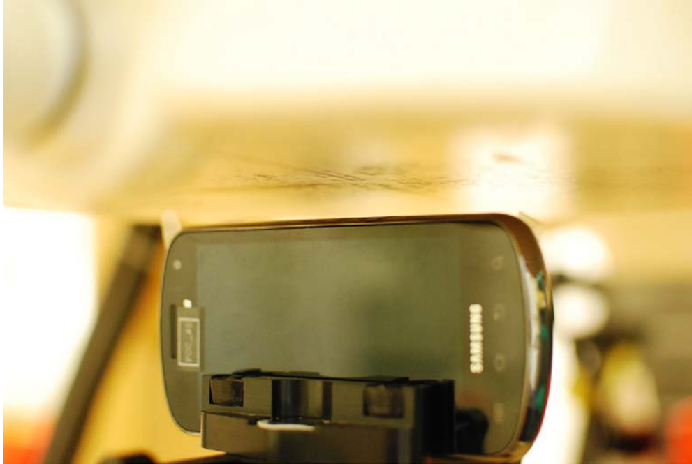
SAR Test Setup Photo 9 – Right at 1.0 cm
