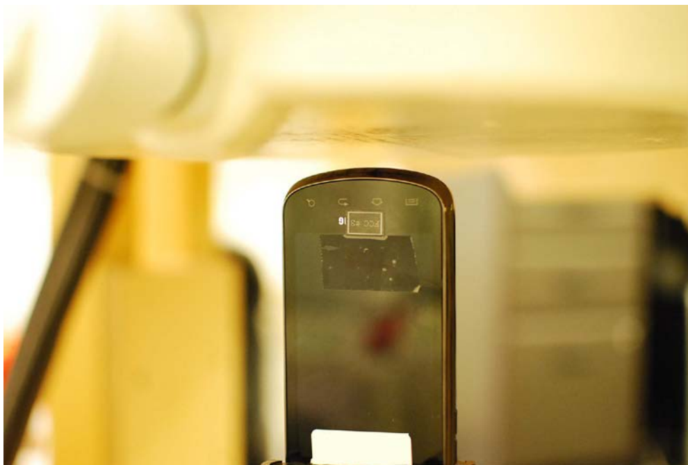
SAR Test Setup Photo 8 – Bottom at 1.0 cm
