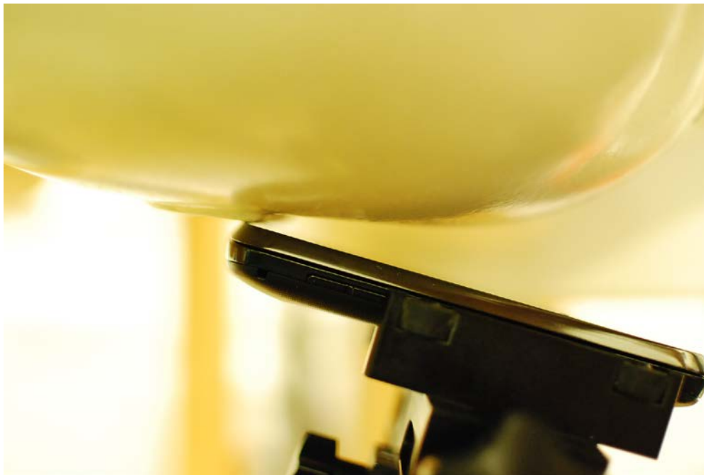
SAR Test Setup Photo 2 – Right Tilt
