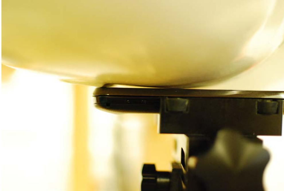
SAR Test Setup Photo 1 – Right Touch
