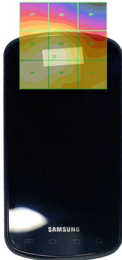
Figure 17-5 H-Field WD Scan overlay
