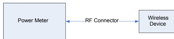
Figure 9-4 Power Measurement Setup
