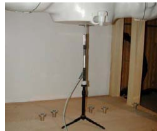
Figure 11-2 System Verification Setup Photo
