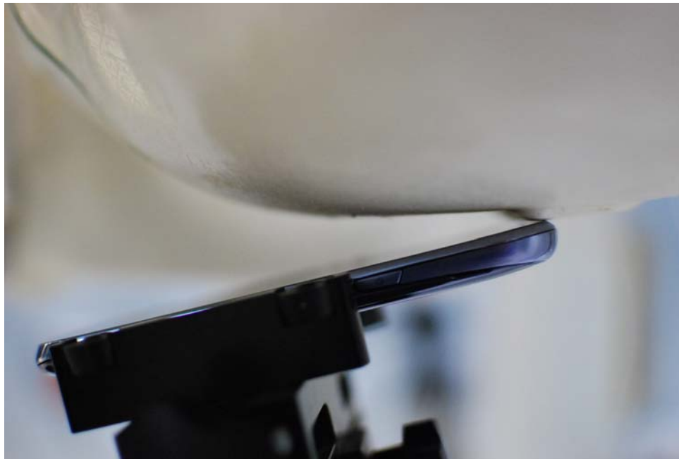
SAR Test Setup Photo 4 – Left Tilt
