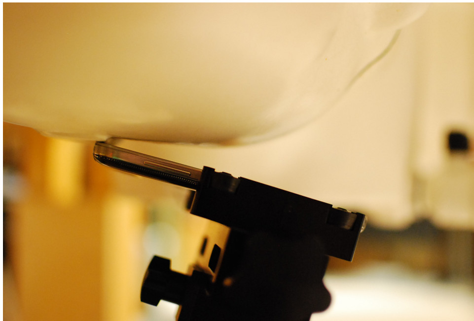
SAR Test Setup Photo 2 – Right Tilt
