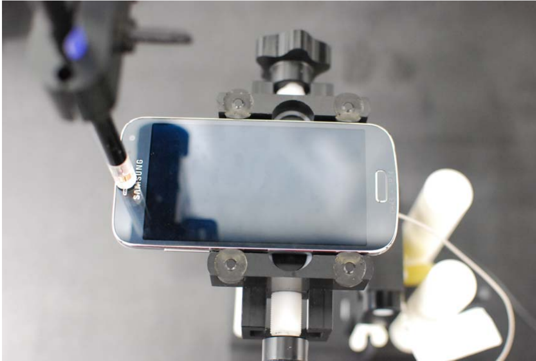
Figure 13-1 Test Setup for Wireless Device
