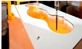
Figure 7-2 SAM Phantom with Simulating Tissue
