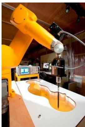
Figure 4-1 SAR Measurement System
