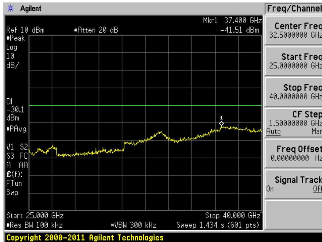
Plot 6-55. Conducted Spurious Plot (802.11a – Ch. 149)
