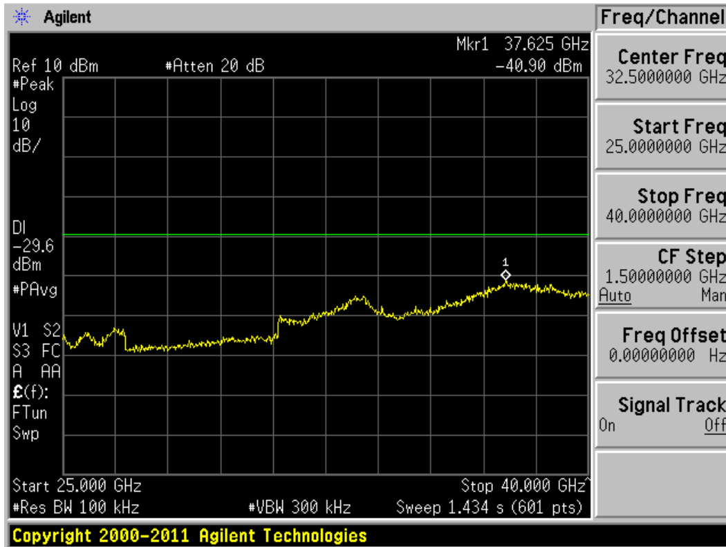
Plot 6-58. Conducted Spurious Plot (802.11a – Ch. 157)
