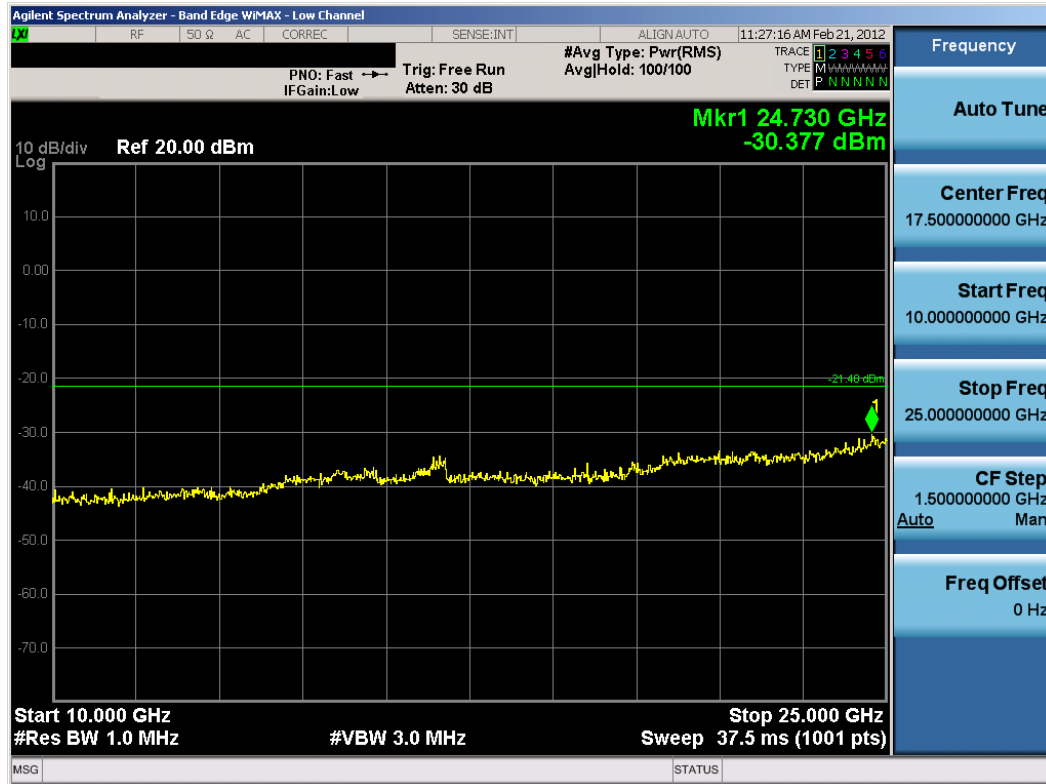
Plot 6-48. Conducted Spurious Plot (802.11b - Ch. 1)
