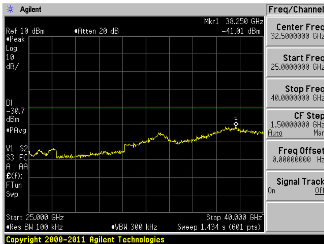
Plot 6-61. Conducted Spurious Plot (802.11a – Ch. 165)
