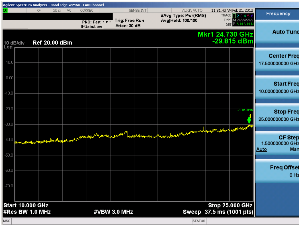
Plot 6-50. Conducted Spurious Plot (802.11b - Ch. 6)
