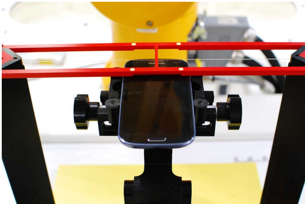
Figure 17-1 Ear Reference Point HAC Phantom Alignment
