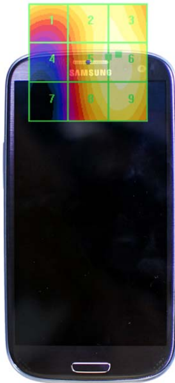
Figure 17-4 E-Field WD Scan overlay
