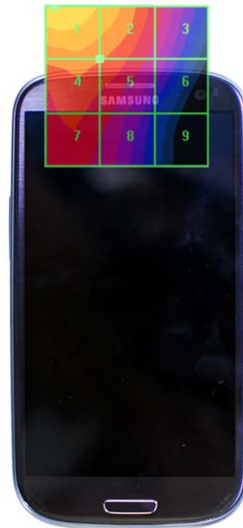
Figure 17-5 H-Field WD Scan overlay
