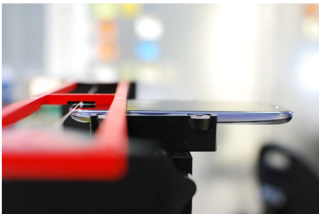
Figure 17-2 HAC Phantom Plane Alignment
