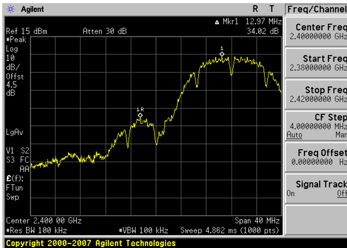
Plot 6-19. Band Edge Plot (802.11b – Ch. 1)
