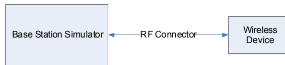
Figure 10-3 Power Measurement Setup
