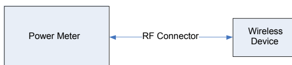
Figure 10-5 Power Measurement Setup
