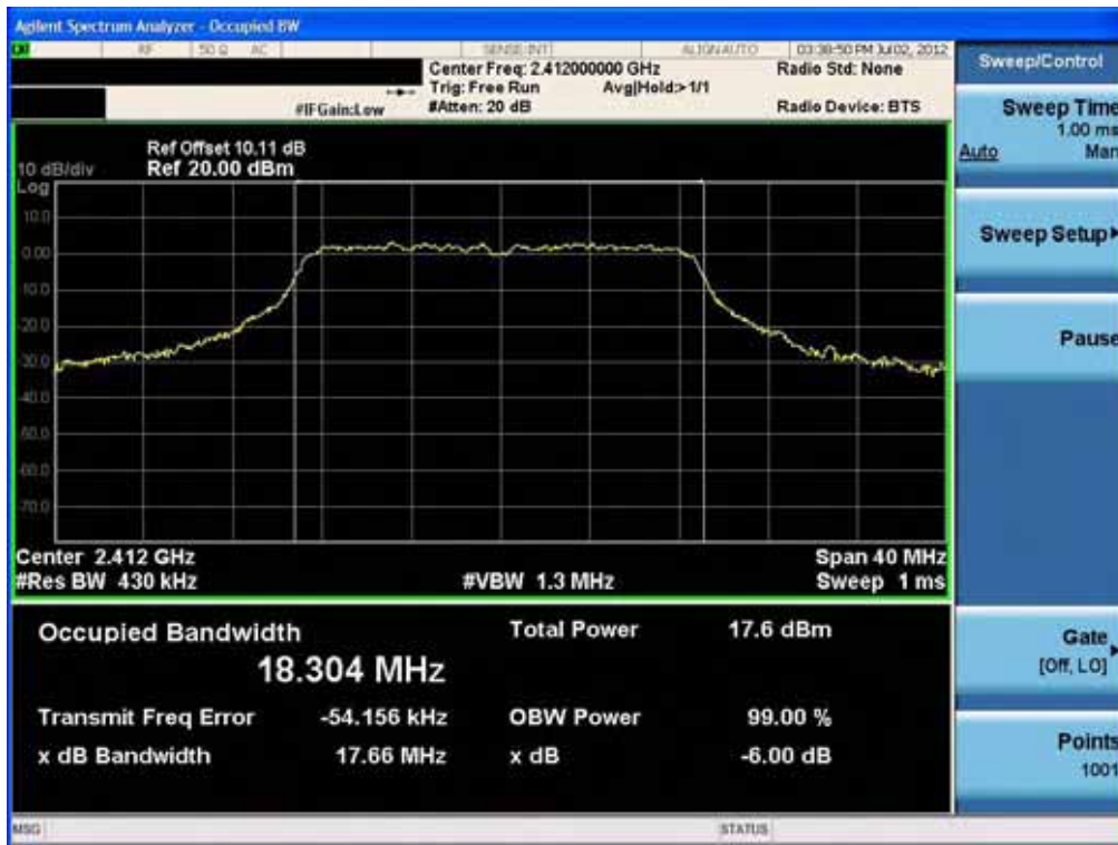
6dB Bandwidth plot (802.11n-CH 6)
