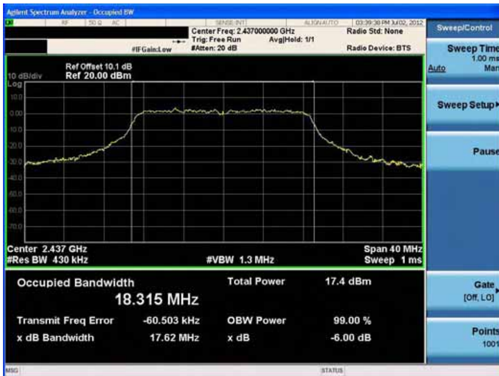
6dB Bandwidth plot (802.11n-CH 6)
