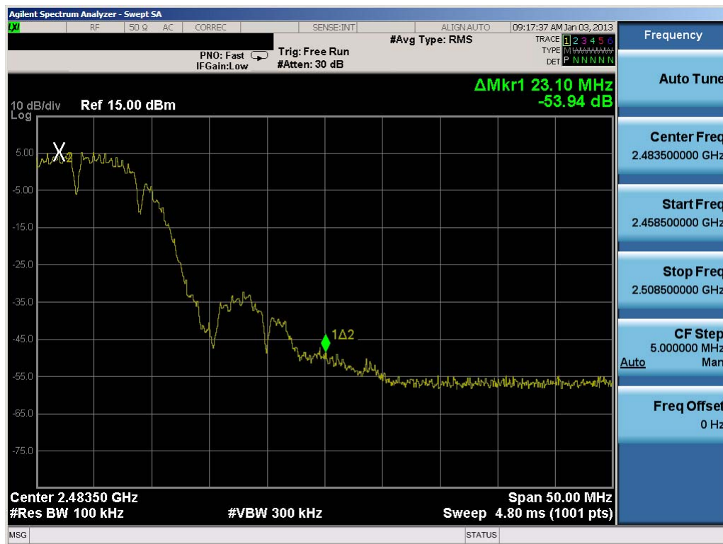
Plot 6-20. Band Edge Plot (802.11b – Ch. 11)
