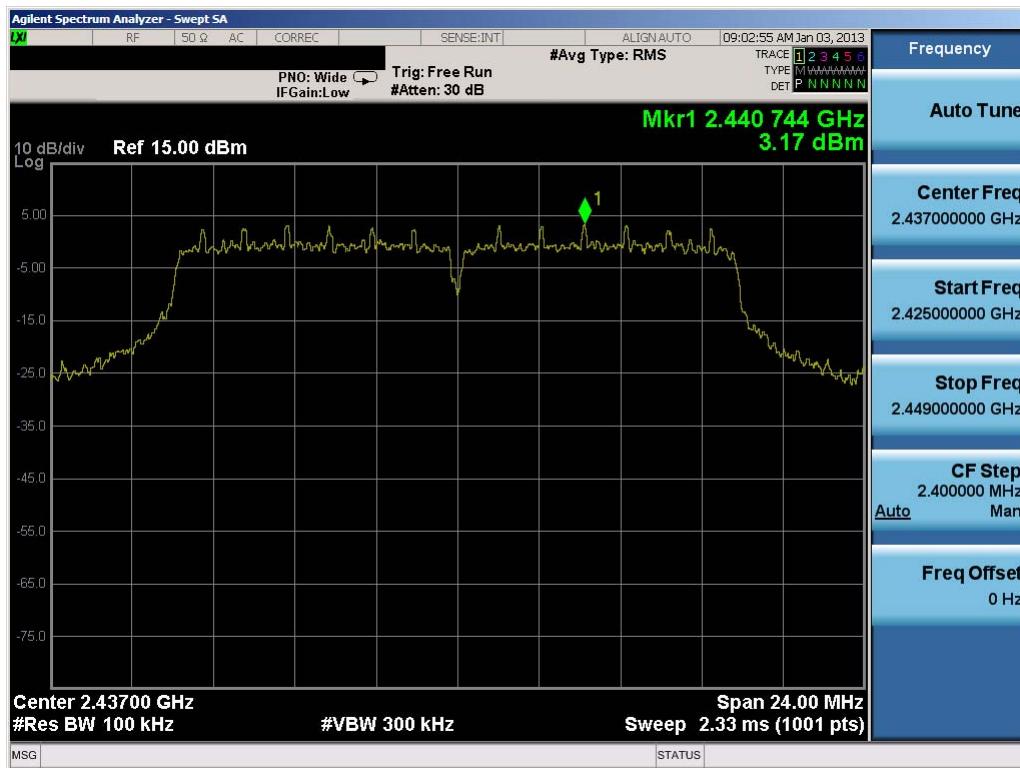
Plot 6-14. Power Spectral Density Plot (802.11g – Ch. 6)
