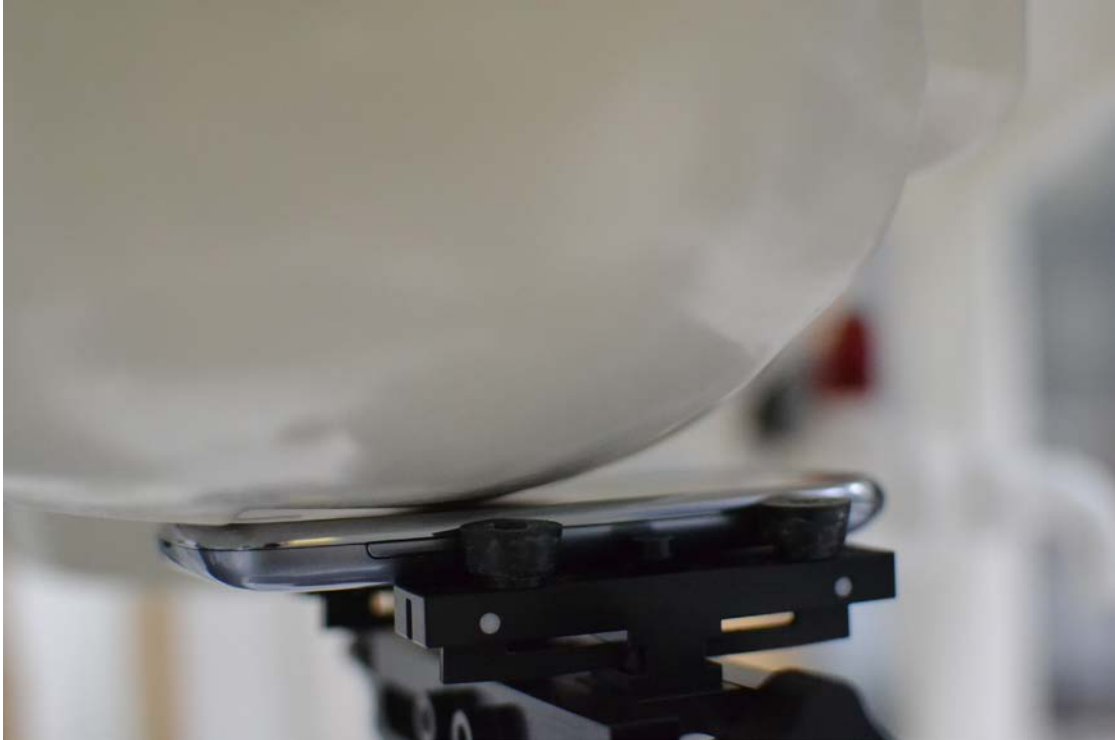
SAR Test Setup Photo 1 - Right Cheek
