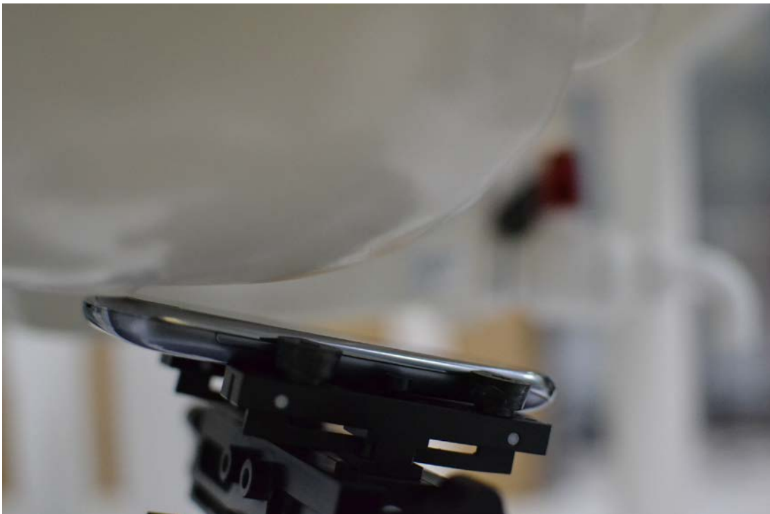
SAR Test Setup Photo 2 - Right Tilt
