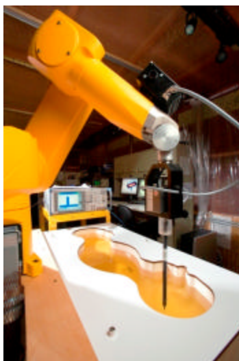
Figure 3-2 DASY4 SAR Measurement System
