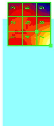
Figure 10-2 Sample H-field Scan Overlay (See Test Setup Photographs for actual WD overlay)
