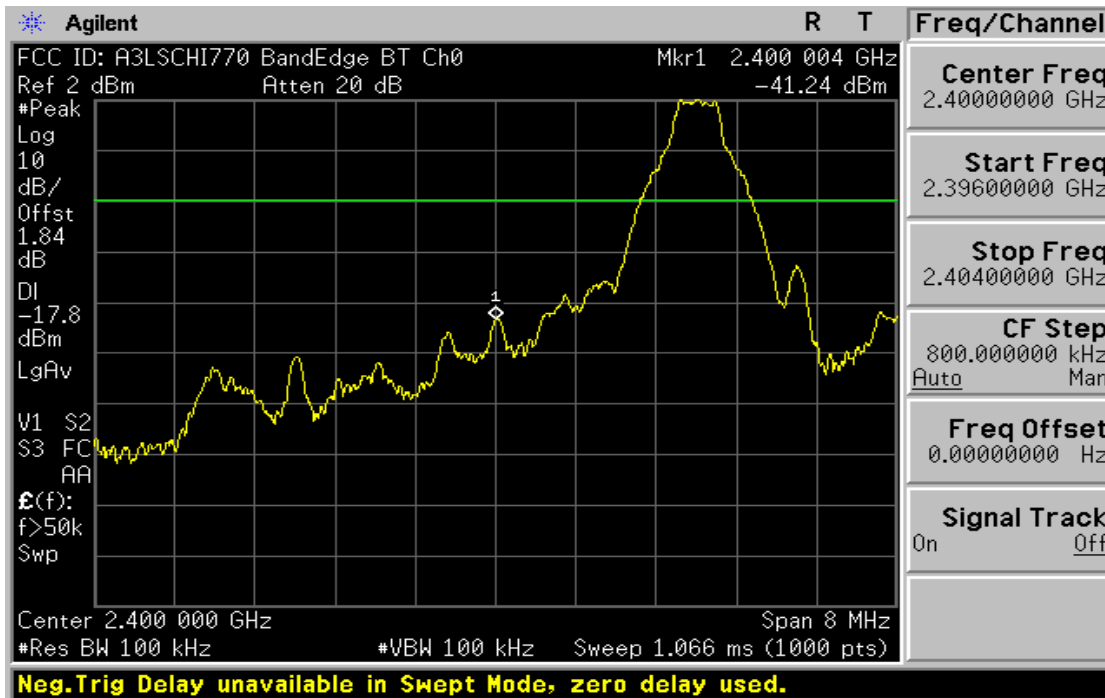
Plot 6-4. Band Edge Plot (Bluetooth – Ch. 0)
