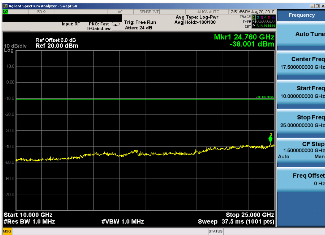
Plot 6-18. Conducted Spurious Plot (802.11b – Ch. 11)
