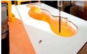
Figure 6-2 SAM Phantom with Simulating Tissue
