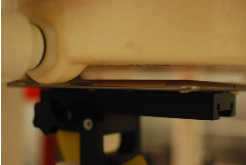
SAR Test Setup Photo 3: Back at 1.0 cm
