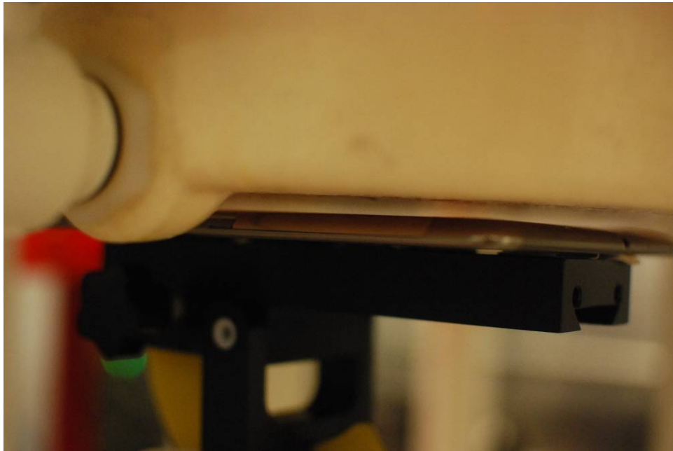
SAR Test Setup Photo 2: Back at 0.5 cm
