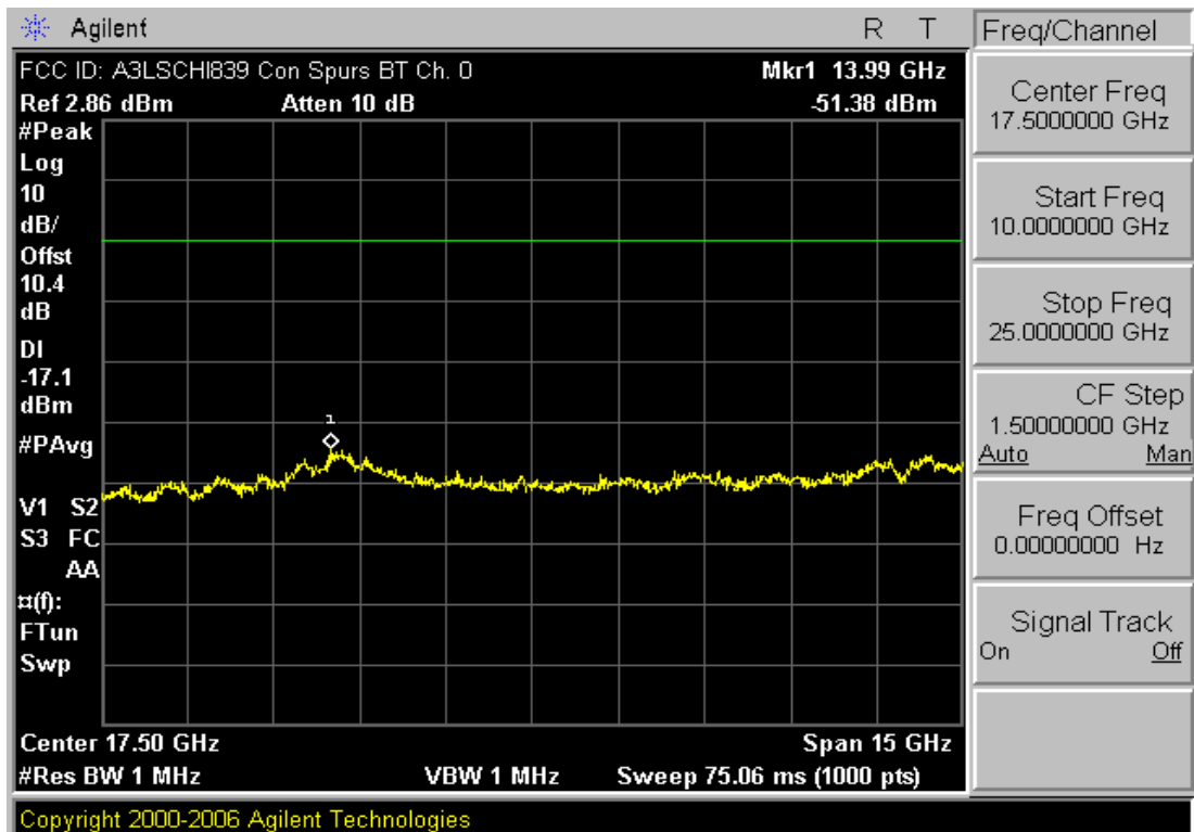
Plot 6-13. Conducted Spurious Plot (Bluetooth – Ch. 0)
