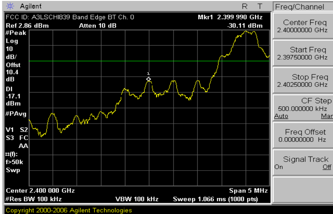
Plot 6-4. Band Edge Plot (Bluetooth – Ch. 0)
