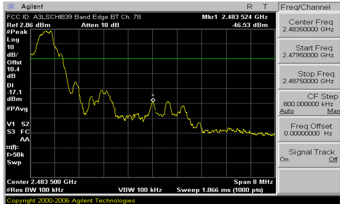
Plot 6-5. Band Edge Plot (Bluetooth – Ch. 78)
