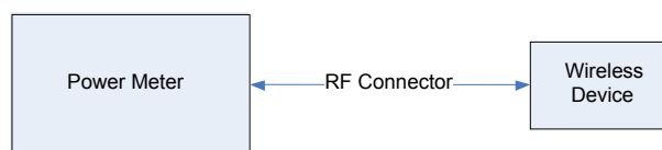
Figure 8-2 Power Measurement Setup
