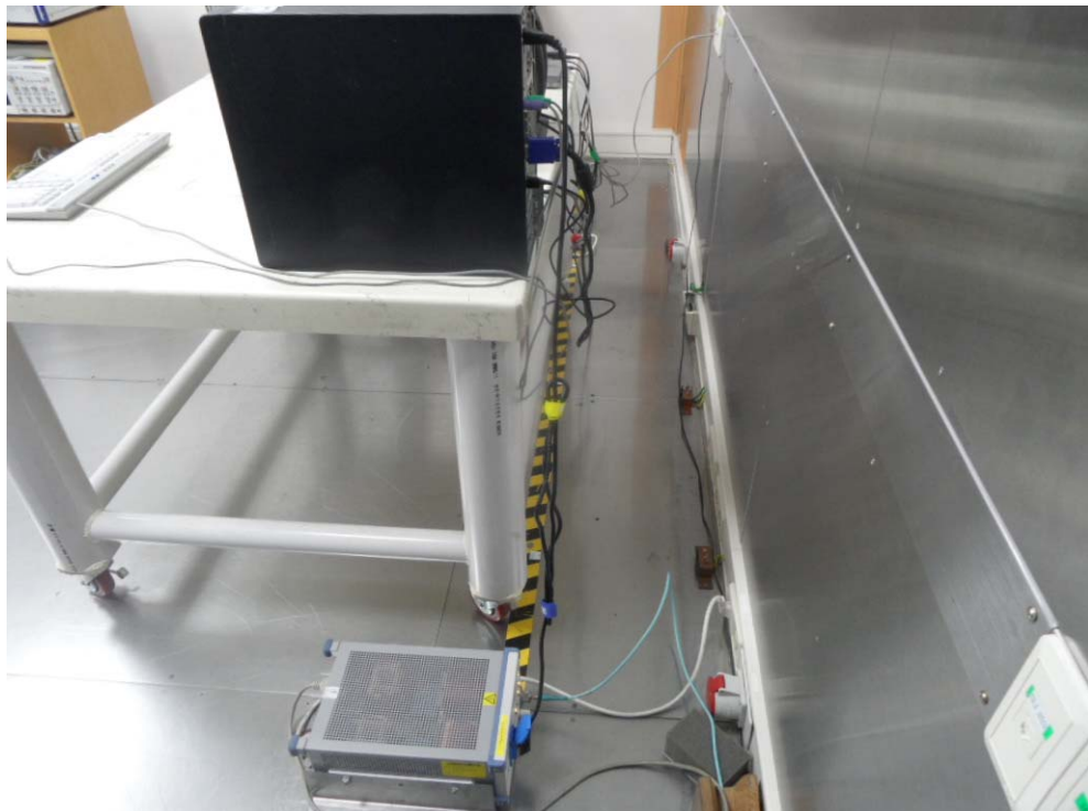
[ Conducted Disturbance – Rear ]
