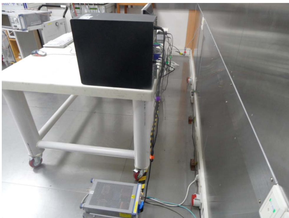
[ Conducted Disturbance – Rear ]
