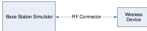
Figure 12-1 Power Measurement Setup
