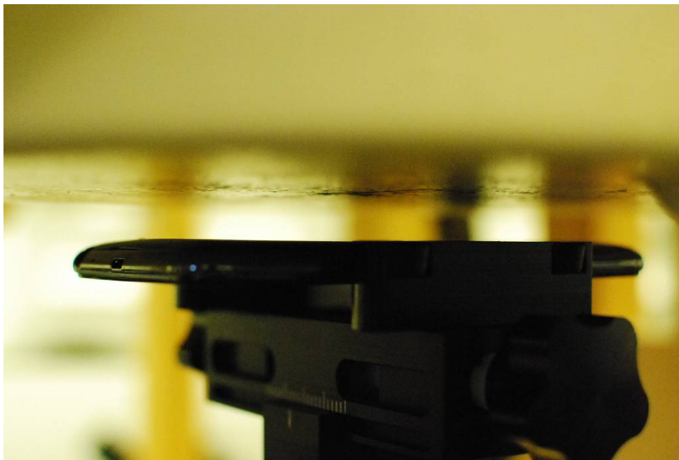
SAR Test Setup Photo 6: Body Back at 1.0 cm
