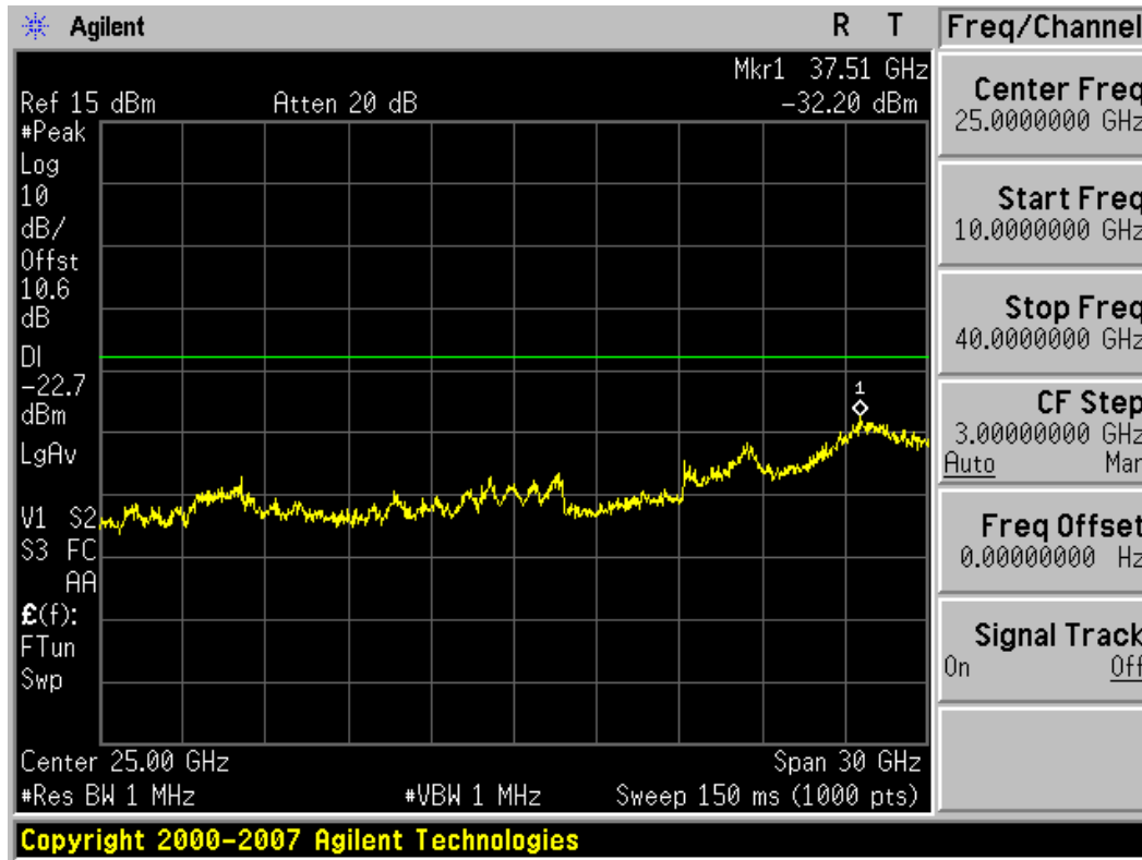
Plot 6-50. Conducted Spurious Plot (802.11a – Ch. 157)
