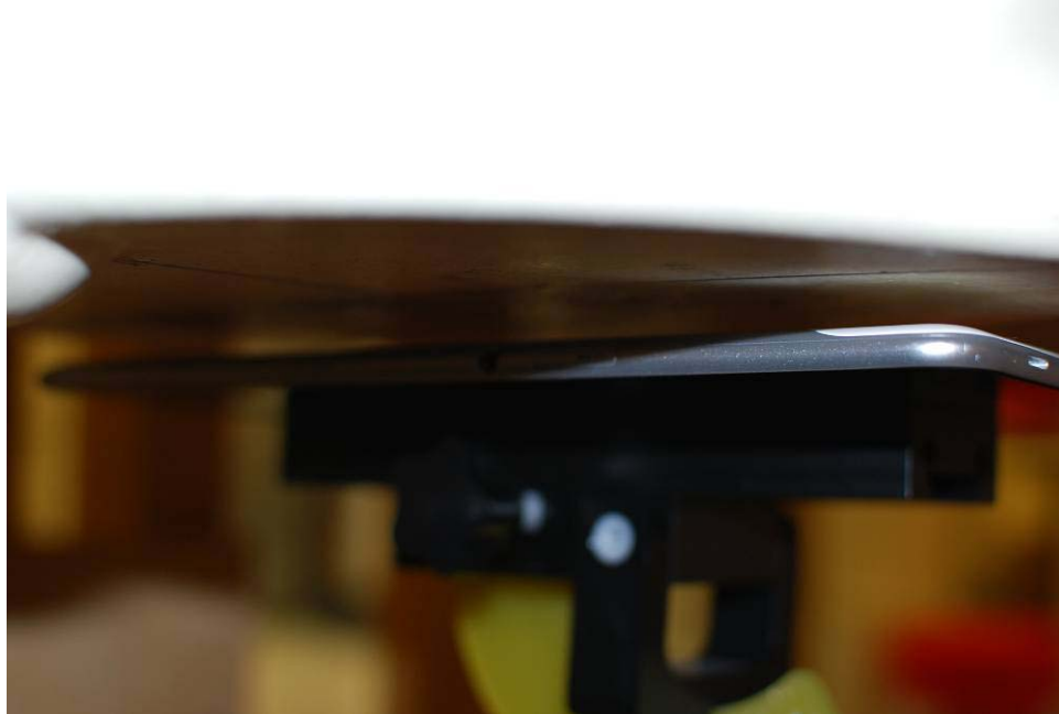
Figure 22-3 SAR Test Setup Photo 3: Back at 1.0 cm
