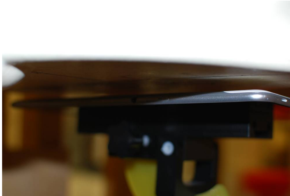
SAR Test Setup Photo 3: Back at 1.0 cm
