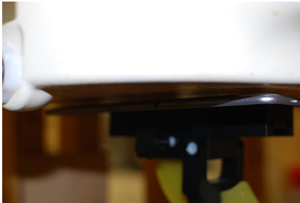
SAR Test Setup Photo 2: Back at 0.5 cm
